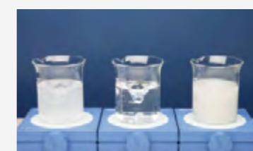
After 20 minutes of stirring, PANACAL L-Calcium Lactate dissolves completely but water remains clear. While the other 2 substances did not dissolve completely, turning the water milky.
